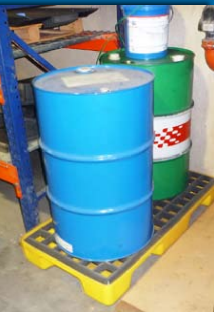
Keep containers tightly covered and positioned on spill pallets. This helps prevent contaminants from leaking onto floors and making their way into the storm drain system.
